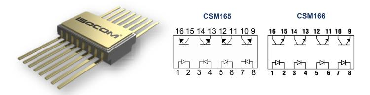
The CSM165 and CSM166 are hermetically sealed, radiation hard optically coupled isolators, composed of a Gallium Arsenide infrared emitting diode and a silicon phototransistor. These electronic components are available in both Dual Channel (CSM165-2 and CSM166-2) and Quad Channel (CSM165-4 and CSM166-4). The CSM165-4 radiation tolerant optocoupler is the Quad Channel version of the IS49.
